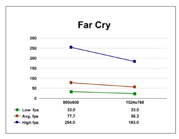
Even on the aging 9800 Pro and its 128 MB of on board memory, Far Cry still turns in very playable frame rates at 1024x768, though testing was conducted without anti-aliasing or anisotropic filtering enabled. A roughly 30% performance drop occurred between the two resolutions.
