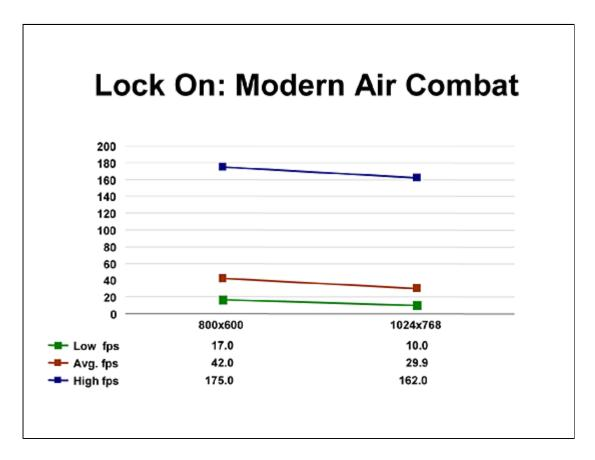
The 9800 Pro is clearly limiting Lock On's performance in this playback, with such a substantial frame rate loss between the tested resolutions. This is the rare flight simulation that scales well with faster graphics boards.
