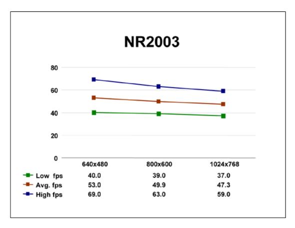
NR2003 appears somewhat CPU-limited, with a roughly 10% variation in frame rate within the range of tested resolutions. These scores, however, are still very high and show the horsepower of the 3800+.
