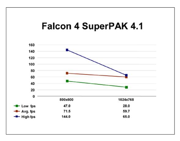
Again we see a fairly significant frame rate loss — in this case roughly 15% — between tested resolutions.
